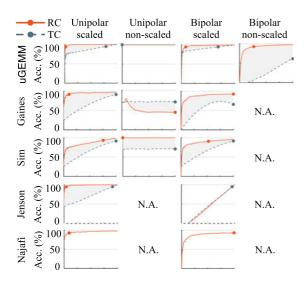
**FIGURE 5.** Progressive accuracy (curves) and stability (dots) comparison of GEMMs. Cycle ranges from 1 to 256 in uGEMM, Gaines,' Sim's and Najafi's; and from 1 to 256<sup>2</sup> in Jenson's. RC: rate-coded input; TC: temporal-coded input.
