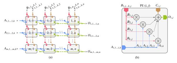
FIGURE 4. uGEMM architecture and its PE. Thick line: multibit stream; and thin line: single-bit stream.
