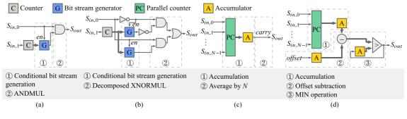
FIGURE 3. uGEMM functional units. Thick line: binary signal; and thin line: unary signal.
